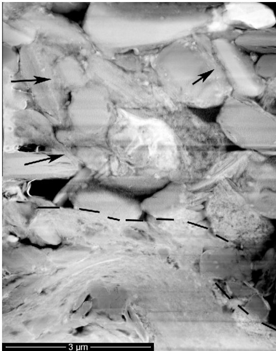
Fig. 6. A FIB section imaged with TEM of Ashikule Basin varnish, Tibet, where area beneath the black dashed line is dominated by the clay–Mn–Fe laminated matrix of rock varnish. Above this varnish-dominated zone is a quartz-rich layer with abundant detritus. We note nanoscale coatings on most of the detrital particles. In many places (e.g. arrows), a mixture of clay–Mn–Fe varnish penetrates into inter-grain areas. This mixed texture of pockets of varnish and detrital minerals is consistent with the movement of capillary water through pore spaces, with subsequent movement of water involved in the precipitation of Mn–Fe remobilized from laminated varnish.
