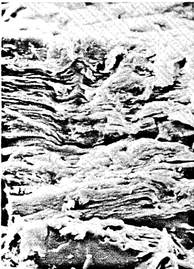
Plate 2: Cross-section of varnish collected from Peparuta Bluff, Oulnina Homestead, South Australia. The parallel lamellate structure indicates abundant clay minerals. Note the distinct morphological break between the underlying rock and the varnish. Width of SEM image is about 40 microns.
