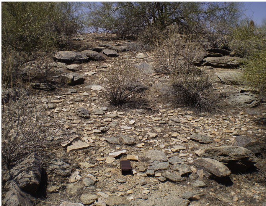
Fig. 4. Typical detachment trap setting very near the crest. Note that the typical armoring by cobbles, boulders and bedrock. Each trap (brown rectangular box) was either attached to a large clast on its underside by superglue, but a few were weighted down with clasts placed inside and then removed after trap collection. A sense of scale is provided by the triangle-leaf bursage ( Ambrosia deltoidea ) plants in the middle of the frame are 0.5 m high.
