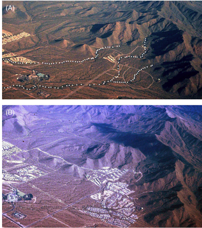
FIGURE 10.16 Development burgeoned on alluvial-fan surfaces during the 1990s, as shown in a comparison of 1991 (A) and 1995 (B) aerial photographs of the southern McDowell Mountains, Scottsdale. In the 1991 image, dots delineate the presence of entrenched channels transporting water and sediment almost 8 km downstream from this fan. Thus, with the hydrological apex located at distance from the topographic apex of the alluvial fan, all of the development is safe from fan-related flooding.
