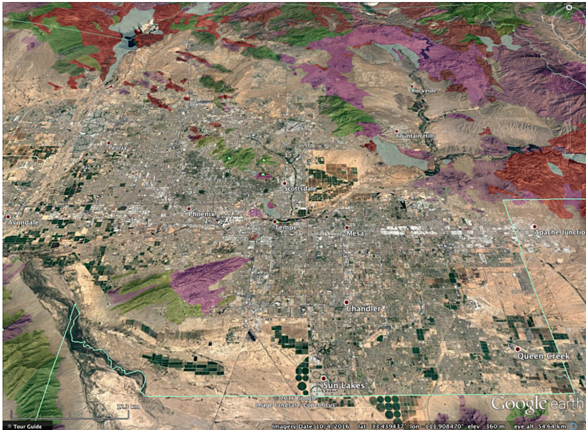
FIGURE 10.2 Geological map of bedrock ranges in the metropolitan Phoenix overlaid on a Google Earth oblique image. The mapping units derive from the Arizona Geological Survey (Richards et al., 2000), but are generalized here to help visualize isolated bedrock mountainous areas: intrusive igneous (pink), extrusive igneous (red), metamorphic (green), and mid-Tertiary sedimentary rocks (gray). Most urban space, thus, rests on Quaternary sediment ranging from Pliocene to Holocene in age. Source: The image is used following permission guidelines for Google Earth to Source: The image has been modified from a Google Earth image ( http://www.google.com/permissions/geoguidelines.html ) with mapping units derived from Richards, S.M., Reynolds, S.J., Spencer, J.E. Pearthree, P.A., 2000. Geologic Map of Arizona. Arizona Geological Survey Map M-35, 1 sheet, scale 1:1,000,000.
