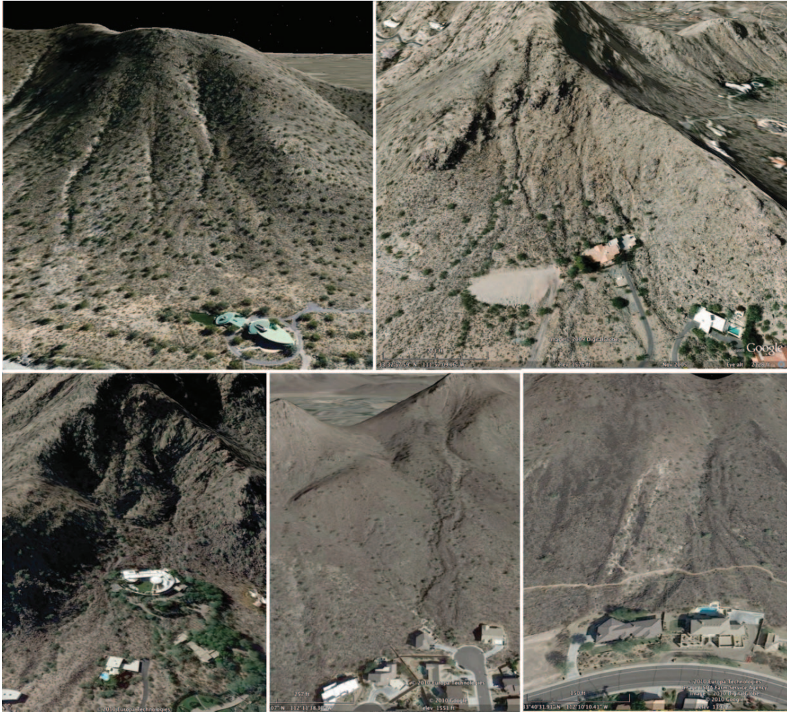
Figure 2 Examples of homes in wealthy mountainside neighborhoods built under debris-flow-generating catchments. The upper left image shows a debris-flow fan near Taliesin West, Scottsdale. The upper right image displays a large home and a future home site under debris-flow channels at Mummy Mountain, Paradise Valley. The lower left image shows homes placed under bedrock channels at Camelback Mountain; the lower middle image from Ludden Mountain illustrates home placement on former debris-flow levees, and the lower right image from Hedgpeth Hills reveal homes placed on a debris-flow fan. These images follow permission guidelines for Google Earth ( http://www.google.com/permissions/geoguidelines.html ). (Color figure available online.)
