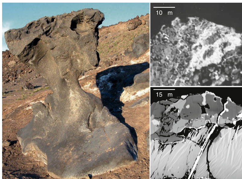
Figure 19 Barium sulfate, sodium chloride, calcium sulfate, and strontium sulfate weathers Mushroom Rock in Death Valley, California. The BSE micrographs on the right show a barium sulfate crust as the brighter material both fragmenting the basalt and covering mineral surfaces. The bright white in these images are barite and darker crystals are weathered basalt silicate minerals.
