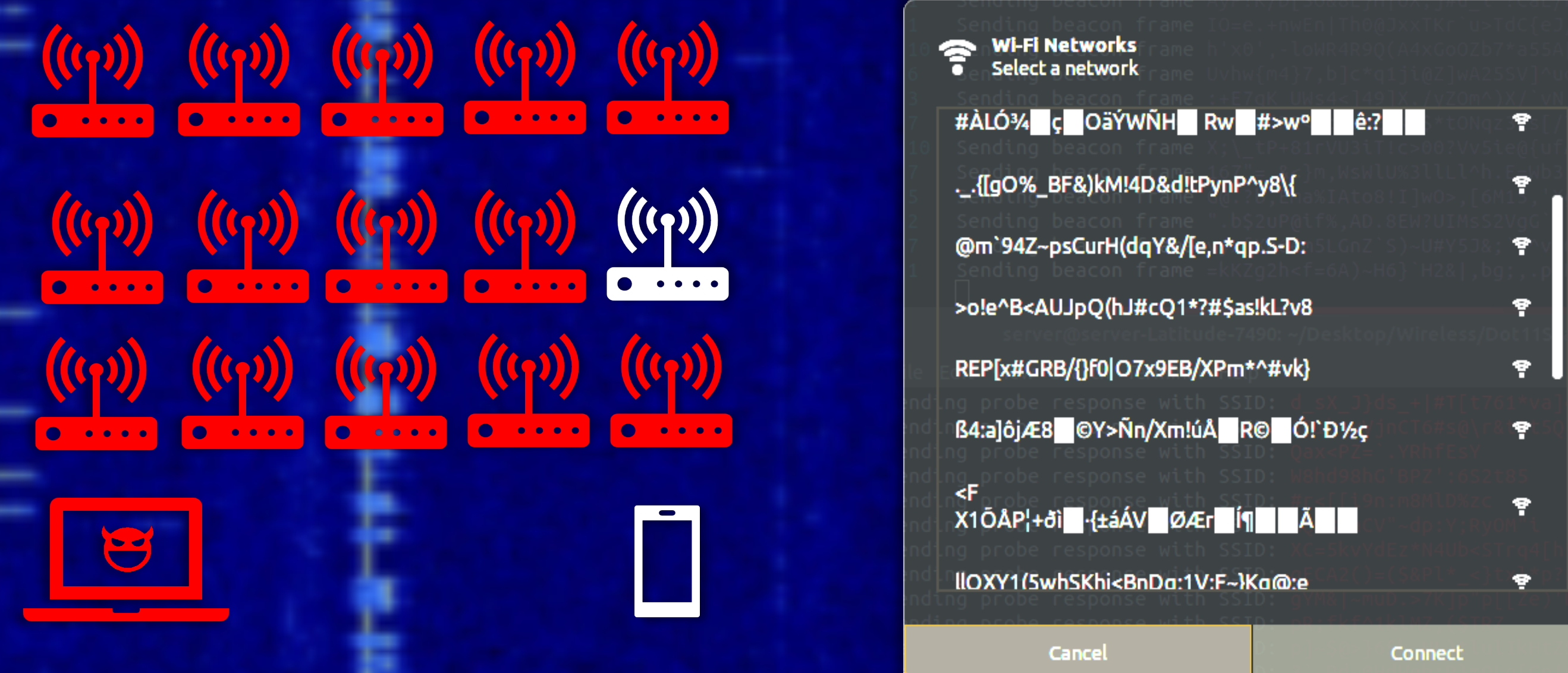
Figure 1 – Attacker creates endless stream of fake access points colored in red. Amongst a single real access point.
