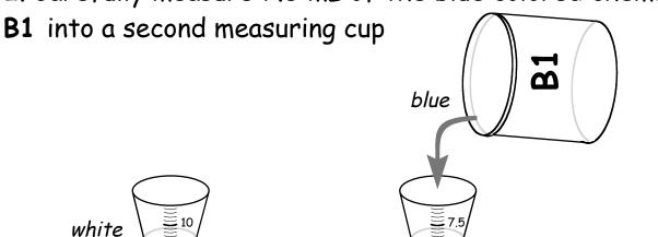
3. Add the 7.5 mL of the blue **B1** chemical to the 10 mL of the white **A1** and stir with a wooden stick
