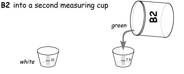
3. Add the 7.5 mL of the green **B2** chemical to the 10 mL of the white **A2** and stir with a wooden stick
