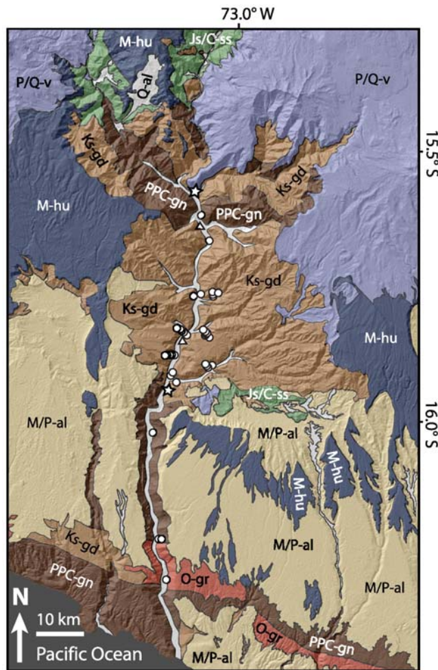
Figure 2. Simplified geologic map of Ocoña canyon based on mapping by INGEMMET [2001] and by Schildgen et al. [2009]. Dated valley-filling volcanic flows are too small to appear at the scale of mapping, but locations are shown with white triangles. White circles indicate thermochronology sample locations. PPC-gn, Precambrian gneiss; J/C-ss, Jurassic/Cretaceous sandstone, limestone; Ks-gd, Cretaceous granodiorite, diorite, and tonalite; M/P-al, Mio-Pliocene alluvium, landslide, and marine sediments; M-hu, Miocene Huaylillas Formation ignimbrites; P/Q-v., Plio-Quaternary extrusive volcanics; Q-al, Quaternary alluvium.
