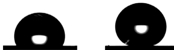
Figure 3. Examples of water drops on surfaces having identical spiropyran coatings and irradiated with visible light: smooth (left) and rough nanowire (right) surfaces.
