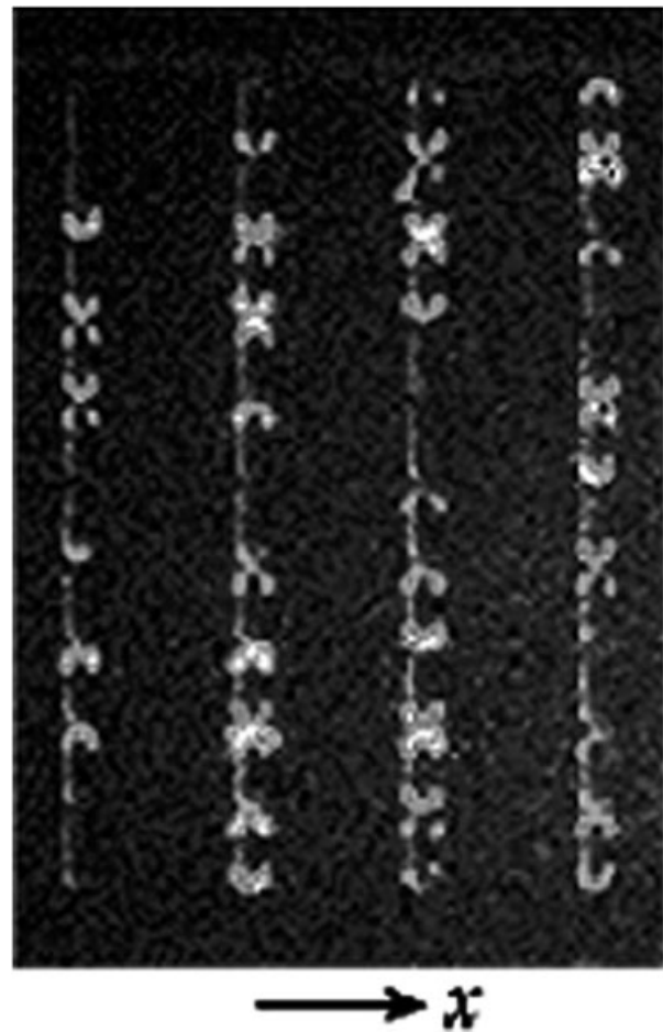
Figure 7. Fluorescence micrograph depicting the DEP entrapment of 164 kbp DNA between posts.
