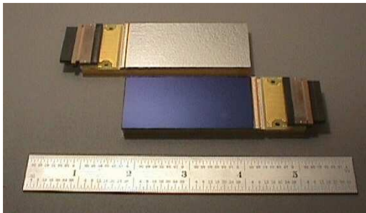
Figure 14: The lower of the above CCDs has had a coating of \text{MgF}_2 applied, while the upper chip is thinned but still without any coating. Courtesy: M. Lesser/UA/ITL.
