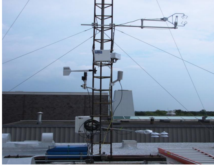
Figure 4.5. Experimental set-up of Sensorscope station over suburban area
