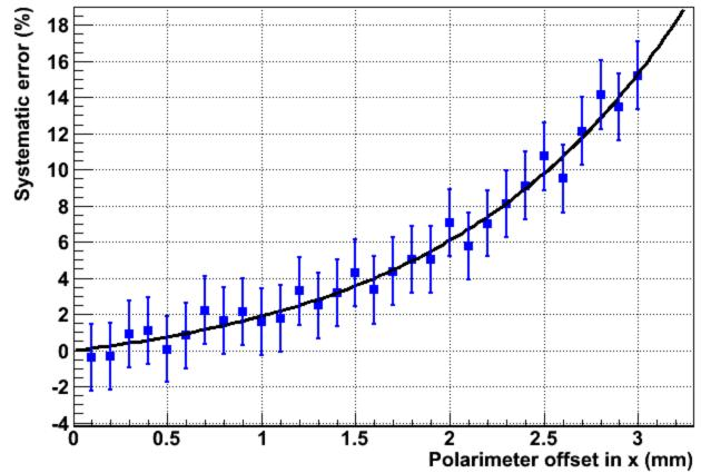
• Alex talked to engineers and they can center the polarimeter to within 200 microns ©
