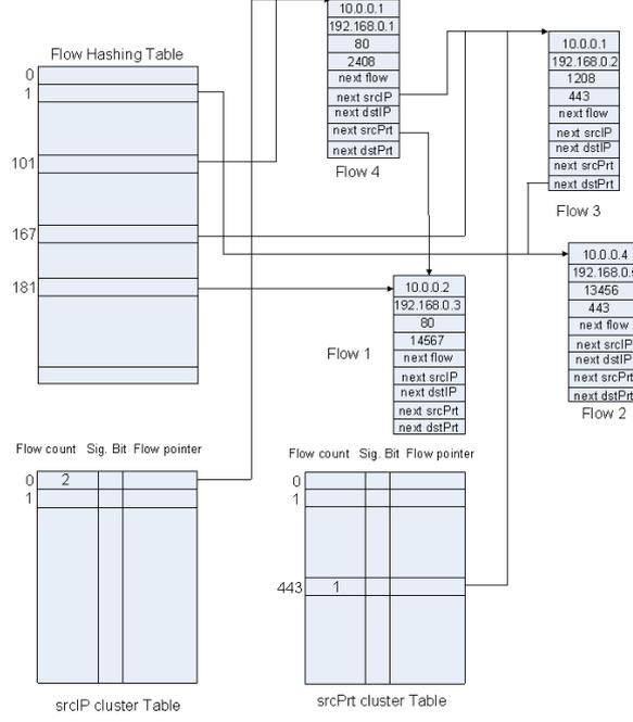
Figure 4: Data structure of flow table and cluster table
