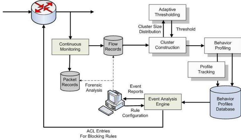
Figure 3: The architecture of real-time traffic profiling system
