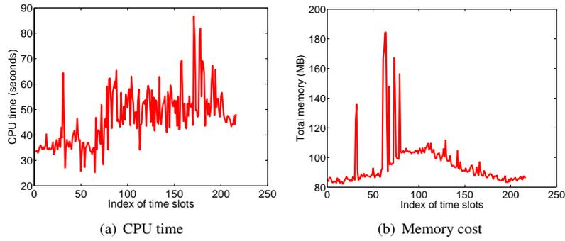
Figure 5: CPU and memory cost of the real-time profiling system on flow records in 5-min time interval collected in  $L_1$  for 18 consecutive hours
