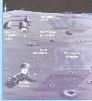
Figure 1. In this lunar power base, sunlight hits the solar converter, which transmits power via underground wires to a microwave generator, which in turn illuminates a microwave reflector. All such reflectors, when viewed from Earth, overlap to form a "lens" that can direct a narrow power beam toward Earth.
