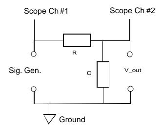
Fig. 4. Experimental setup used for the determination of the decay constant of an RC circuit.
