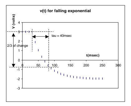
Fig. 3 Quantitative example showing v(t) exponentially falling from +3 to -2 volts with a time constant of 40msec, starting at t0=30msec.
