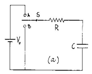
Fig. 1. Schematic of RC circuit with charge/discharge switch.
