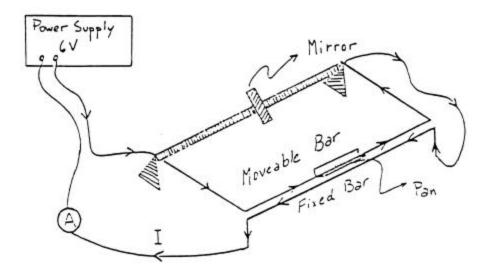
Fig. 1. The current balance apparatus.
