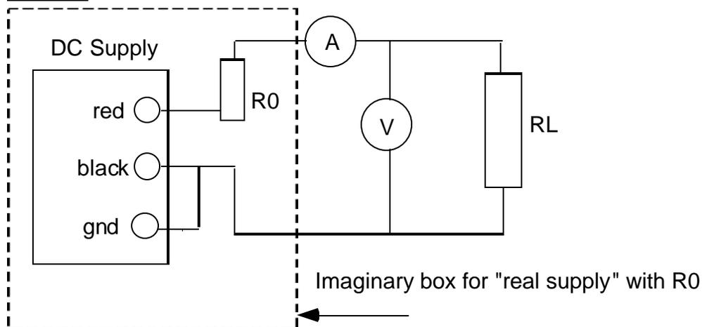
Figure 1. Circuit for measuring power in load resistor.
