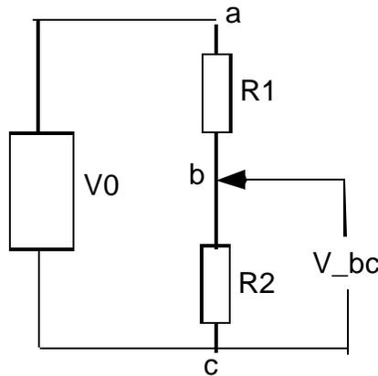
Fig. 2 Potentiometer shown as a voltage divider.
