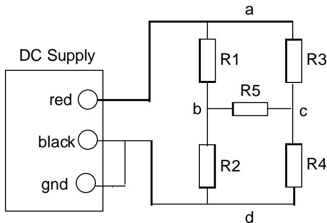
Figure 1. Wheatstone bridge circuit.
