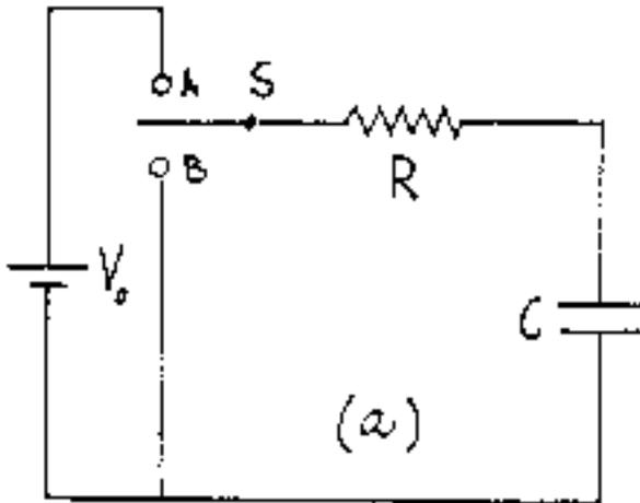
Fig. 1. Schematic of RC circuit with charge/discharge switch.
