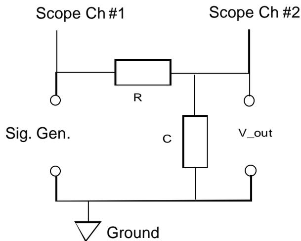
Fig. 4. Experimental setup used for the determination of the decay constant of an RC circuit.
