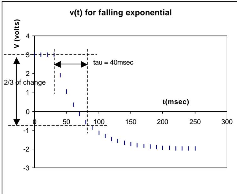
Fig. 3 Quantitative example showing  $v(t)$  exponentially falling from +3 to -2 volts with a time constant of 40msec, starting at  $t_0=30\text{msec}$ .
