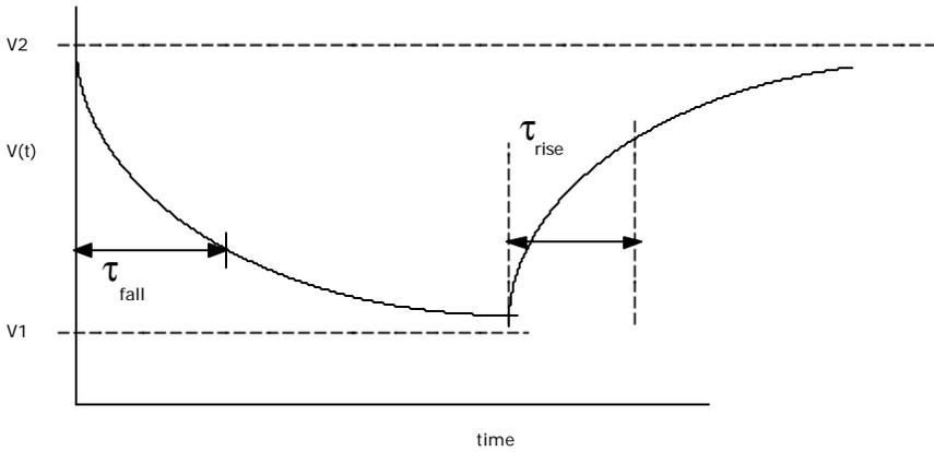
Fig. 2 Illustration of eyeball method to extract time constant for either falling or rising exponential relaxation.
