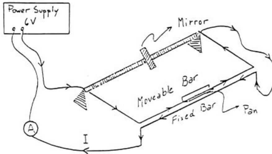
Fig. 1. The current balance apparatus.
