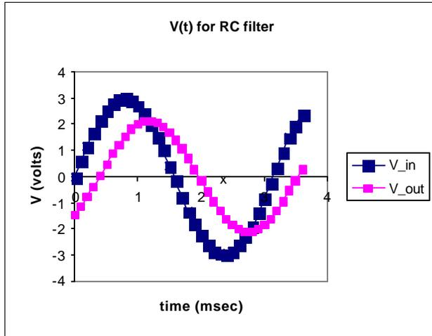
Fig. 2 Sample  $v(t)$  waveforms for RC filter.
