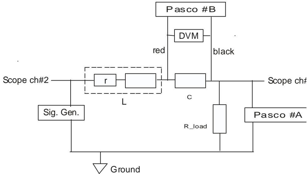
Fig. 3 Circuit used for measuring LRC behavior.
