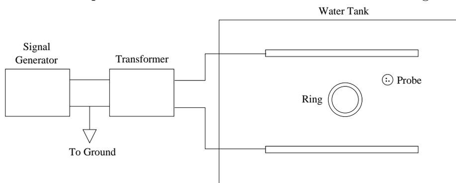
Part (1a): Create the set-up shown in the figure, but don't use the metal ring; there should be a piece of graph paper under the tank from which you can read coordinates. Use the signal generator ( $f = 200$  Hz, amplitude maximum) to generate an AC signal
