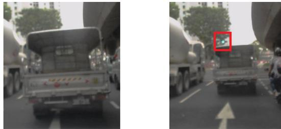
Fig. 1: Example of traffic light occlusion by other vehicles. The light is obscured in the left image but becomes visible in the right image as the traffic starts moving.
