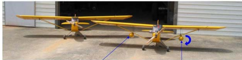
Deployable POD ( Robotic Agent, Sensor , Beacon, Landmark etc.)
