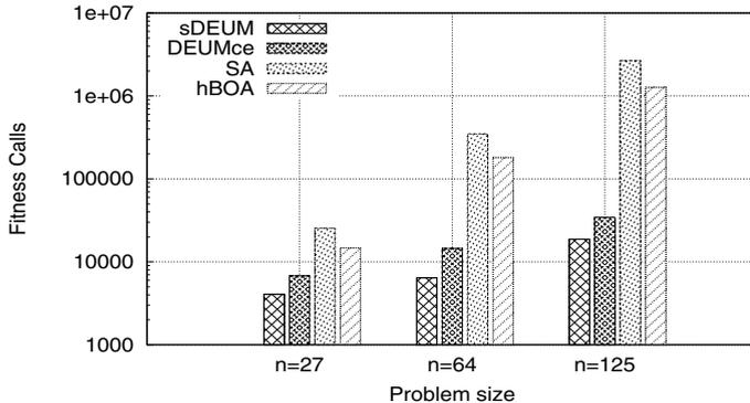
**Fig. 3.** Average number of evaluations of  $f$  (log scale) over problem size required to find first optimal solution with probability 1. Benchmark: 3D Ising Spin Glass function,  $n \in \{27, 64, 125\}$ . Algorithms: sDEUM, DEUMce, SA, hBOA.
