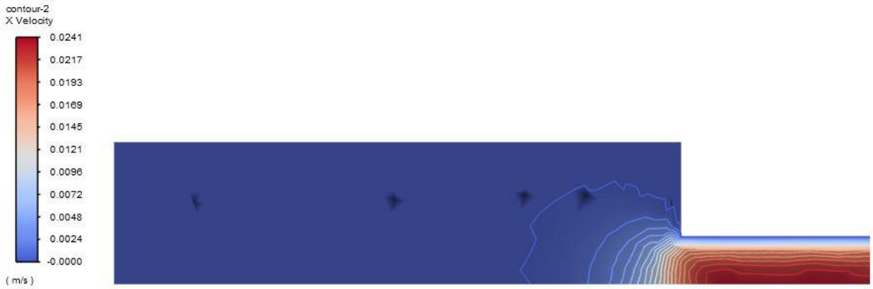
Figure 23. Contour Plot of Velocity on the Vertical Plane of Symmetry for Quarter Model
