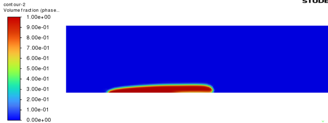
Figure D8.3: Plane of symmetry contour plot of glycerin volume fraction at t = 0.2 s
