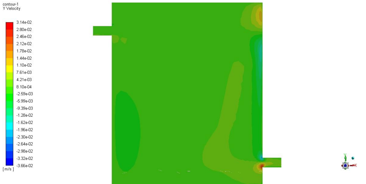
Figure 9. Y-Velocity contour plot for task # 2
