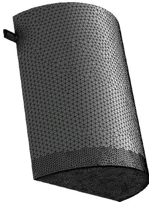
Figure 1. Isometric view of geometry and mesh generation of the half-cylinder water tank.
