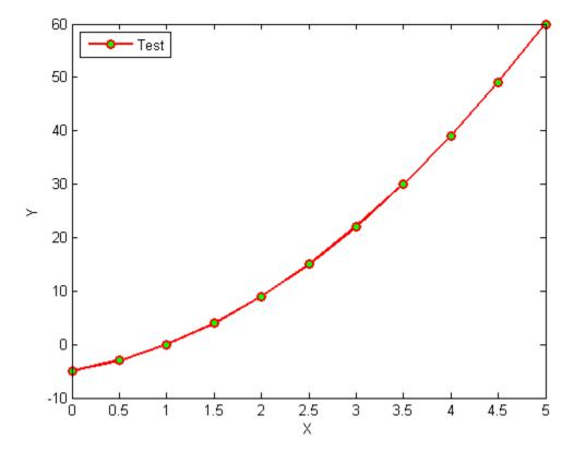
Remarks: The '-or' in the *plot* command set the line pattern. In this case, it's solid line with circular symbol. The circular symbol is filled with green color ('g' for 'MarkerFaceColor'). The legend of the plot is set to locate at teh upper-left corner ('Location'' set to 'NorthWest') inside the frame.
