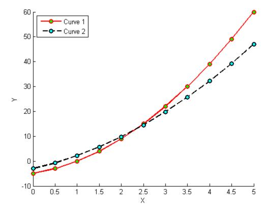
Remark: Without the "hold on" command, the second *plot* will override the first one and acts to erase the curve produced by the latter.
