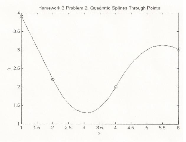
Note: This is the solution with y'' = 0 at  $x_1$ . An alternative solution using y'' = 0 at  $x_4$  is also acceptable.
