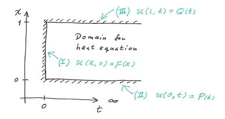
Step 1: Separation of variables. Let u(x, t) = G(x)H(t), the usual procedure leads to
