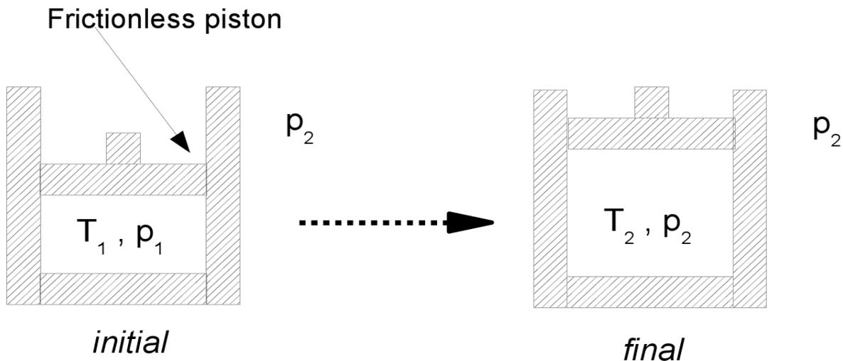
Hint and remarks: (1) While there are different approaches to solve this problem, the most straightforward is to consider that entropy (inside the chamber) is conserved in the process. (2) The outcome of this exercise is relevant to the process of convection and the determination of the vertical temperature profile for the atmosphere, as we will discuss later.
