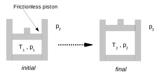
Hint and remarks: (1) While there are different approaches to solve this problem, the most straightforward is to consider that entropy (inside the chamber) is conserved in the process. (2) The outcome of this exercise is relevant to the process of convection and the determination of the vertical temperature profile for the atmosphere, as we will discuss later.
