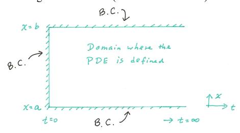
Here, the three boundary conditions (I), (II), and (III) have to be satisfied at the three "walls" at bottom, top, and left, respectively.
