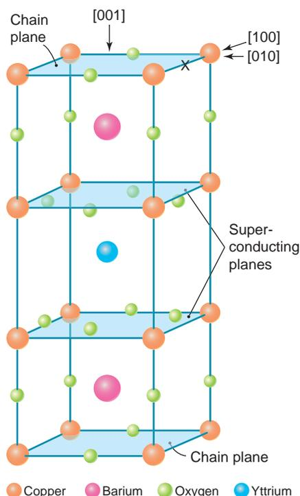
**Oxygen starvation.** Jia *et al.* (1) have obtained atomic-resolution views of the  $\text{YBa}_2\text{Cu}_3\text{O}_7$  superconductor crystal along the three directions shown, allowing them to identify missing oxygen atoms such as those at X. These oxygen vacancies control superconducting properties.
