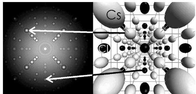
FIG. 2. Left: Multiple scattering produced by point sources of 1 MeV electrons on Cl atoms in a thin film of CsCl (7 monolayers thick). Each blob in the figure lies over an atomic position in the perspective diagram of the crystal structure shown at right. The source atom lies above the plane of the paper and is not shown.
