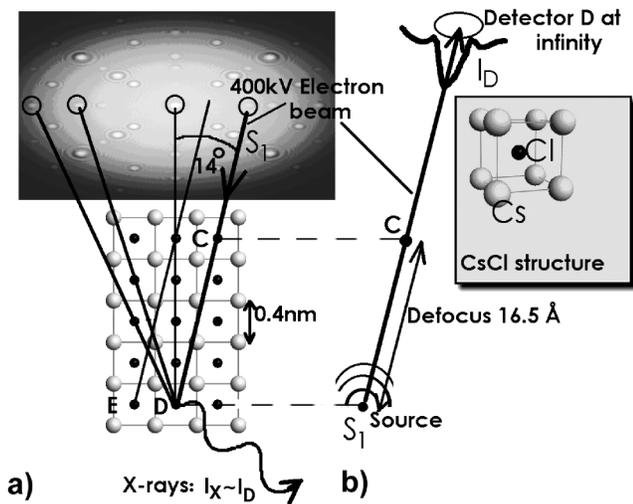
FIG. 1. Atomic-string holography at high electron energies. (a) Incident beam running along atomic columns excites fluorescence, whose total yield is mapped above as a function of incident beam direction. Atomic columns corresponding to spots in the pattern can easily be identified. (b) Time-reversed point source of high energy electrons produces similar pattern. Inset shows CsCl bcc structure.
