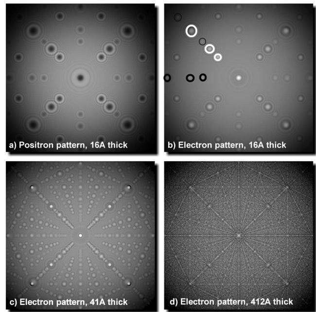
FIG. 3. (a) 1 MeV positron hologram. (b)–(d) 1 MeV electron holograms for samples of different thicknesses. The displayed intensity is the sum of holograms due to sources at every depth up to the sample thickness. In (b) the different holograms of Cs and Cl atoms are indicated by white and black circles, respectively (compare with Fig. 2 for position of all the holograms).
