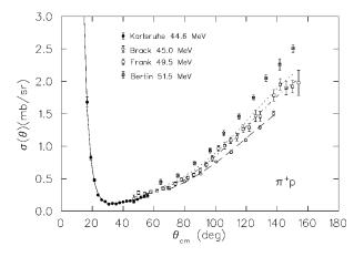
FIG. 1. Cross sections from  $\pi^+$  proton scattering around 50 MeV. The Bertin data would agree with the prediction given by the dotted curve if they were consistent with the other data sets. The solid, long dash and dash-dot curves come from our fit and correspond to the Karlsruhe, Brack, and Frank data sets.
