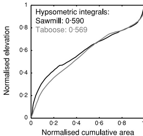
Figure 9. Hypsometric curves for Sawmill Creek (black) and Taboose Creek (grey) in the eastern Sierra Nevada (Figure 2a). Sawmill Creek enters the Owens Valley through a narrow canyon, whereas Taboose Creek has a more typical fluvial V-shaped cross-section. This is reflected in Sawmill Creek having a much smaller proportion of the basin at low elevations
