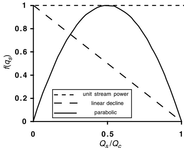
Figure 2. Illustration of postulated models of the  $f(q_s)$  term in equation (1).
