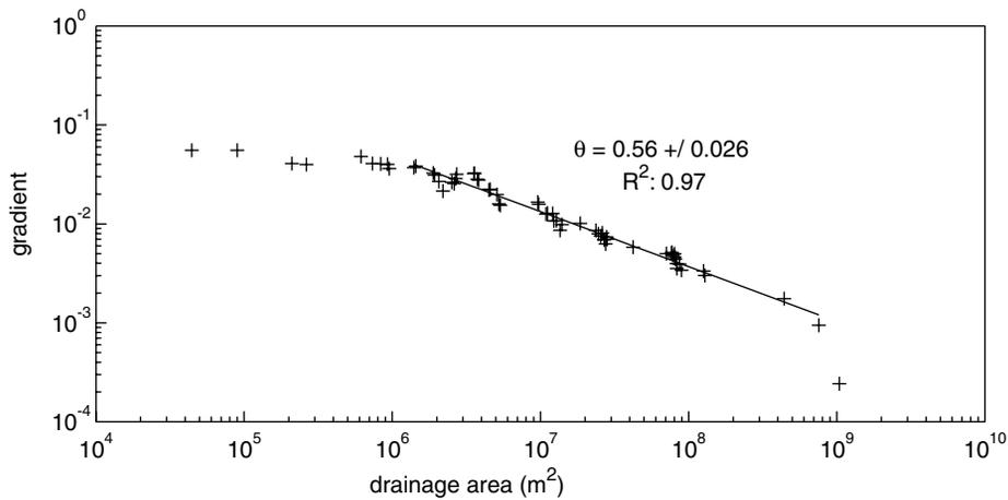
**Figure 5.** Slope-area data for the middle branch of the North River, Virginia (studied by *Hack* [1957]). Break in scaling at  $\sim 10^6$  m<sup>2</sup> may reflect a transition to debris flow-dominated erosion [*Montgomery and Foufoula-Georgiou*, 1993; *Stock and Dietrich*, 1998].
