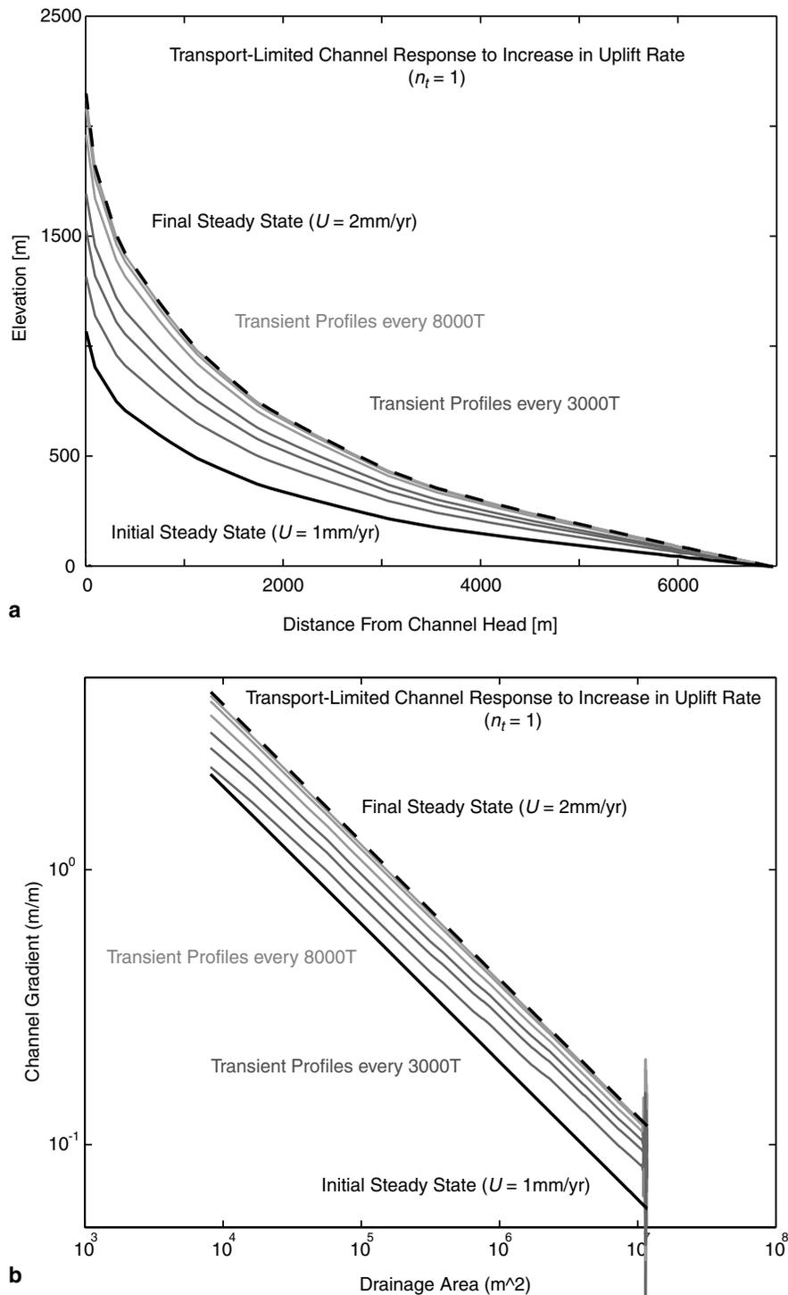
**Figure 8.** Transient response of a transport-limited channel to an increase in rock uplift rate ( $U$ ), shown for the case  $n_t = 1$ . (a) Longitudinal profiles. (b) Channel gradient versus drainage area (log-log scale). Note that the channel evolves by a gradual steepening at an ever decreasing rate (difference from a detachment-limited channel is most evident in Figure 8b). Response time is  $\sim 40,000T$  (model time steps).
