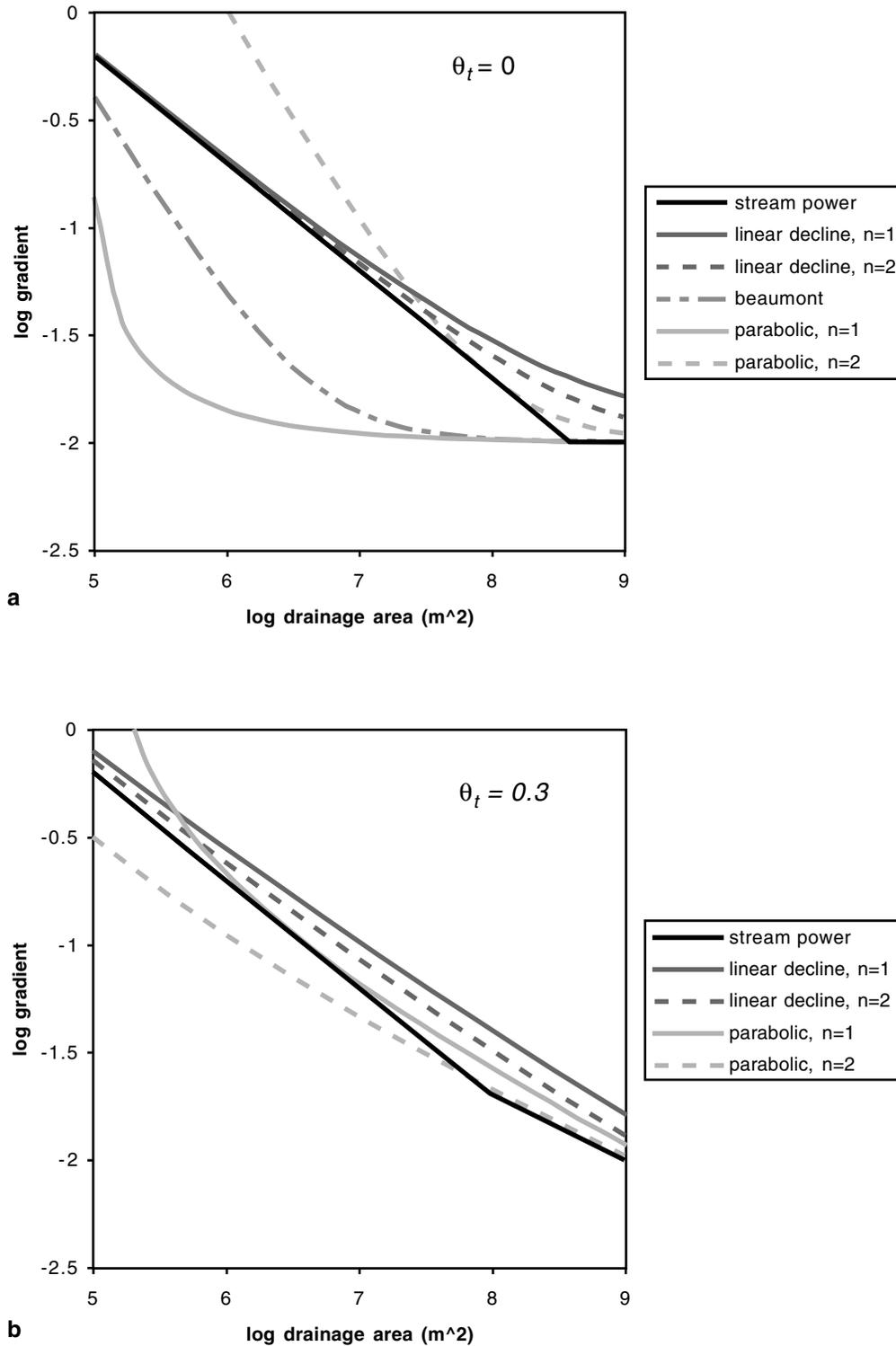
**Figure 3.** Steady state slope-area relations for various  $f(q_s)$  models, with  $\theta_d = 0.5$  and  $n_t = 1$  (bed load transport) assumed in all cases. The parameter  $\theta_t$  crudely represents varying degrees of downstream fining. (a) Relations for  $\theta_t = 0$  (no downstream fining). (b) Relations for  $\theta_t = 0.3$  (significant downstream fining). For  $\theta_t = \theta_d$  all curves collapse to linear parallel lines.
