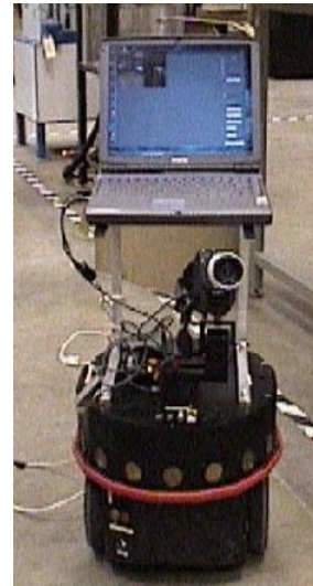
Figure 1: An extra computer is added to the Nomad Scout for image processing. A new program, DVRobot is written which can capture and analyze images from 1394 Digital Cameras or DV Camcorders.
