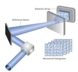
In order to read the data, the reference beam deflects off the hologram thus reconstructing the stored information. This hologram is then projected onto a detector that reads the data in parallel. This parallel read out of data provides holography with its fast transfer rates.
