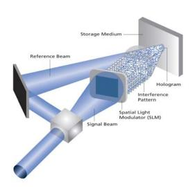
Light from a single laser beam is split into two beams, the signal beam (which carries the
