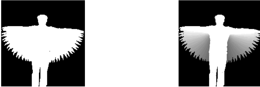
Fig. 7. Temporal templates similar to [34]. Left: Motion Energy Image of a sequence of a person raising both hands, Right: Motion History Image of the same action.
