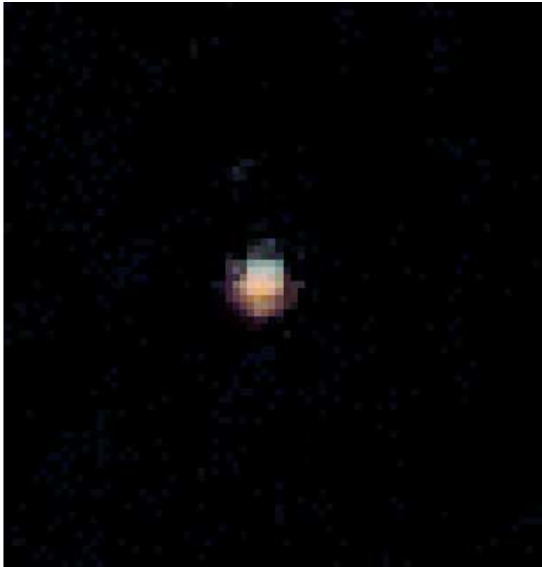
Figure 5: Example of the effects of atmospheric dispersion. The stellar image above was observed in a quick succession of BVR exposures at the 6.5 m Magellan ‘ Baade ’ telescope with the IMACS instrument in Dec 2003 (R. Jansen & R. Windhorst) — before the atmospheric dispersion corrector was commissioned. The air mass was 1.33 (i.e., z \simeq 41^\circ ) and the seeing 0''.75 (3.38 pixels) FWHM. Atmospheric dispersion caused a noticeable differential shift of the centroids of the B and R images on the CCD of \sim 1''.0 .
