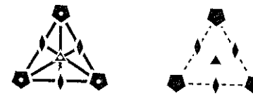
Fig. A4.9. Some of the icosahedral symmetry elements. On the left 2, \bar{5} and \bar{3} axes of I_h are shown with heavy lines representing the traces of mirror planes. On the right are shown the corresponding 2, 3 and 5 axes of I .
