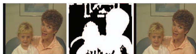
a) Original b) Saliency Map c) Deinterlaced Figure 2. Original frame, saliency map and deinterlaced output
