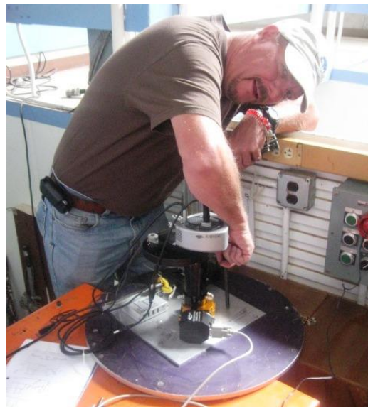
Figure 8. Smith fastens our camera to the large-diameter interface plate for the monsoon engineering checkout.
