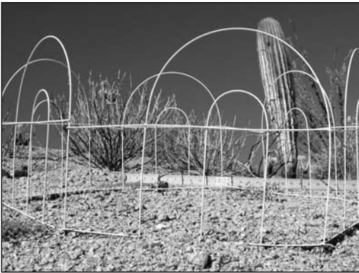
Figure 6. Examples of a two-dimensional understanding of rainsplash transport was measured by placement of a gate system on randomly selected inter-rill slope convexities. Our assumption was that such a slope position would be the location of rainsplash detachment (Parsons et al. 1994).
