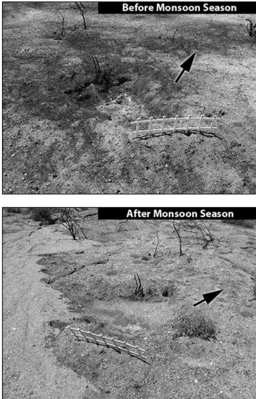
Figure 7. Depressions created by burning of desert scrub roots provided opportunities to measure sediment transport through surveying the dimensions of the depressions. The arrow indicates true north, and the meter-fence provides scale. The top photo pre-dates the summer monsoon (July 15, 2005, just after the fire); the bottom photo represents the same location after the end of the first post-fire Arizona monsoon (October 2005).
