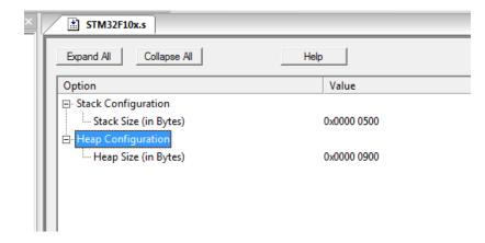
After this modification, make sure that project is rebuilt so that the object generated from the assembler startup file is up to date. This is required because C++test will use this object to complete the build of the final test executable (*objects generated from C/C++ source code are produced by C++test but all the objects generated from assembler files are taken from the original project*).
